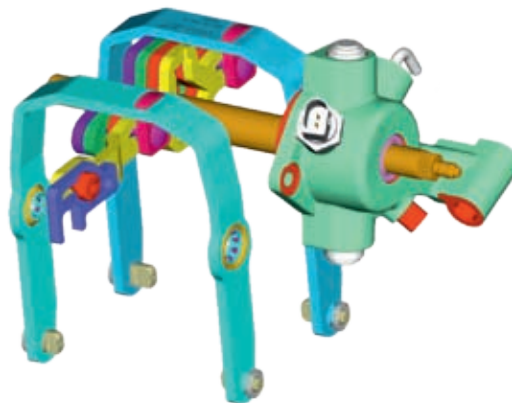
Inner gearshift: The shift fork (blue) and the gearshift dome (green) together constitute the inner gearshift, which is the transmission between gearshift lever and gearbox. The perfect interplay of all components provides for a smooth changing of gears using a gearshift that transmits an ideal torque to the wheels.
