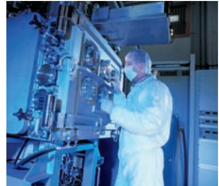
PACVD equipment integrated in a clean room for high purity DLC coatings
