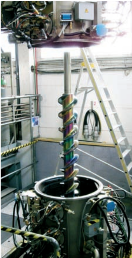
This system technology allows the coating of parts with lengths up to 4,500 millimetres (left and above) and large-volume parts with diameters up to 1,500 millimetres and heights up to 1,800 millimetres (middle and right).
